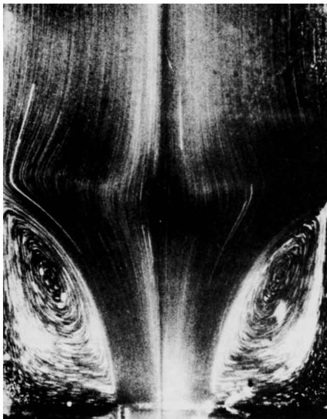
Fig. 4. Flow pattern upstream of the 4:1 contraction for fluids F14 at 154 cm 3 /s, showing divergent flow. ( N_{Re}' = 127 , N_{WS} = 0.483 , 1/5 s at f/8).
