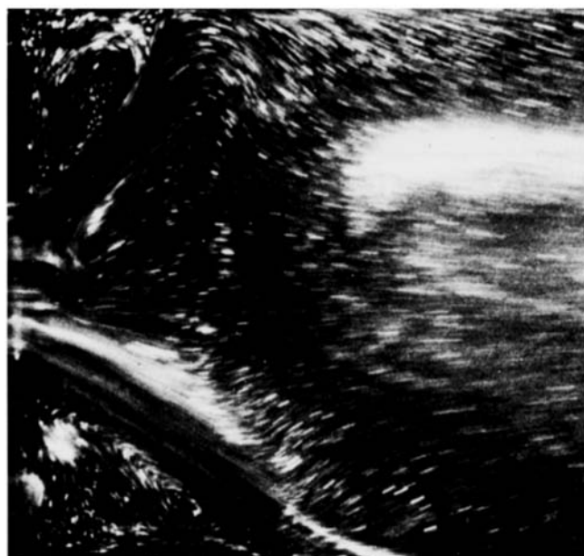
Fig. 8. Flow patterns upstream of the 4:1 contraction for fluid F14 at 550 cm 3 /s, showing random flow distortions. ( N_{Re}' = 886 , N_{WS} = 0.829 , 1/100 s at f/2.8 .)
